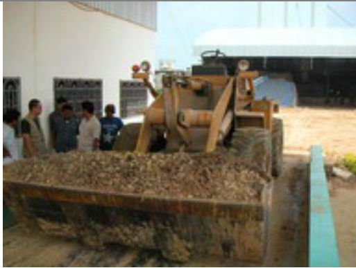
Picture 7: Weighing 1m 3 of corn cobs to estimate density
