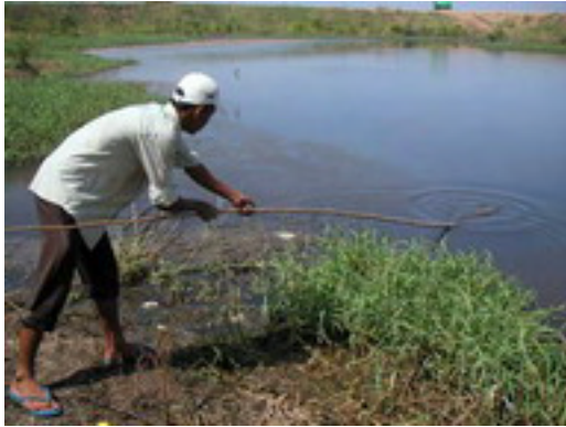
Picture 13: Collecting effluent sample from lagoon
