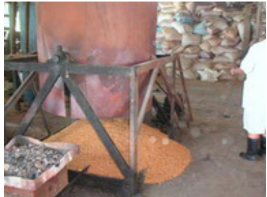
Picture 10: Coal-fired kettle drum for roasting soy beans for feed
